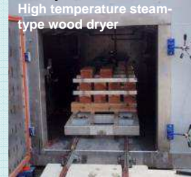
High temperature steam-type wood dryer Development of the drying technology for quality improvement
